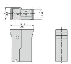
Blanking piece for Power-D-Box (circuit breaker types 8340, 8345)
